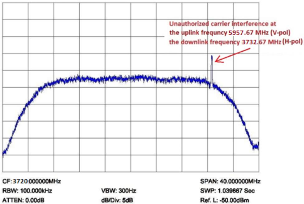
Attachment 2: Downlink plot of A5-CXH (100.5 deg E) centered at 3732.67 MHz
