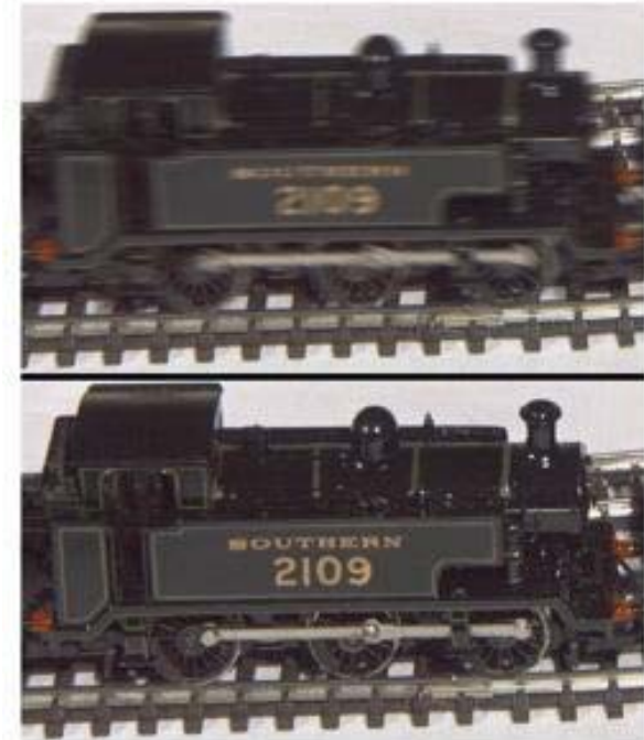
Figure 3. Still from BBC test shoot, above as it would have been captured with 50 Hz frame rate, and below, at 300 fps.
